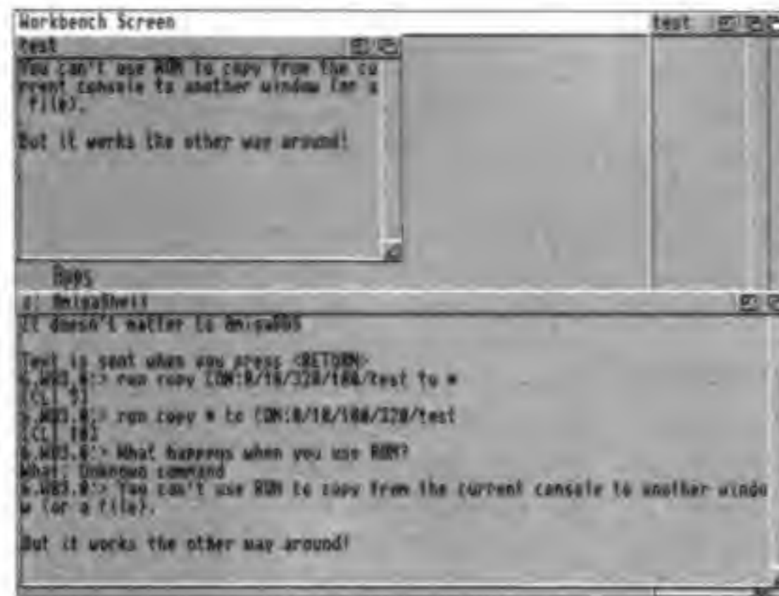
Attempting to combine the two procedures, copy FROM and copy TO, using RUN like this doesn't quite work. The FROM operation gets lost along the line...
